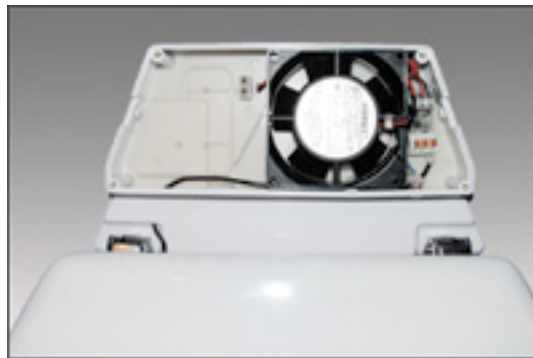
Figure 9: Aspidor Seat Interior (Suction Fan and Microprocessor Chip, which is connected to the red and black wires.)
