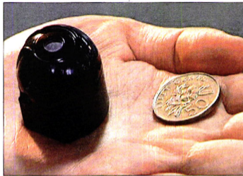
PORTABLE: The i-Ball is a 2-megapixel video camera that does remote video capture and live streaming. (PHOTO: INTERNET)
